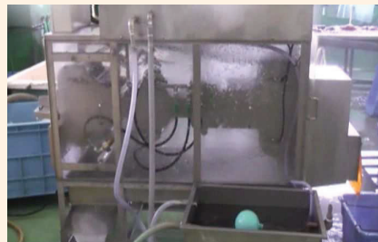
8か所から高圧水が噴射! Hi-pressure water being sprayed out from originally-designed 8-piece nozzle unit
